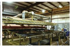
MANTL offers complete refurbishing of your rod inventory. Once your rods arrive at our facility, the team will remove the previous guides, inspect the rods visually or via EMI, clean them, repair any issues, repaint and install new guides. The rods can be shipped back to you or stored in MANTL's yard for future use.
