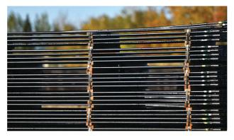
MANTL supplies a full line of sucker rod and drive rod for any artificial lift application.
