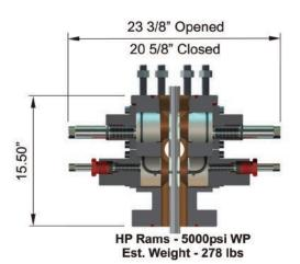
INTEGRAL PRODUCTION BOP WITH POLISH ROD CLAMP 3 1/8" - 3000# TOP & BOTTOM CONNECTION WITH 3 1/2" - 8RD EUE LIFT THREAD
